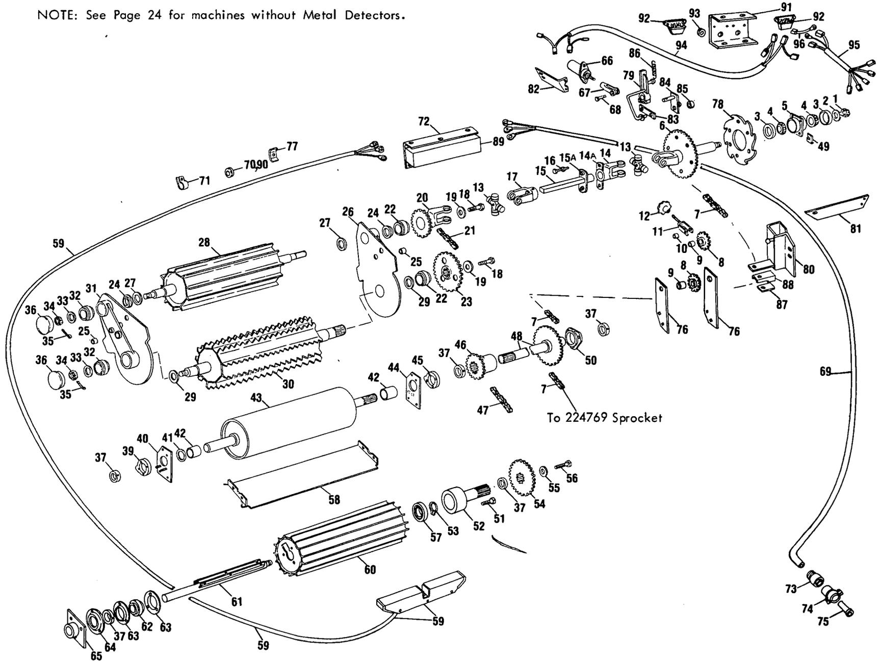
FEED ROLL GROUP FOR MACHINES EQUIPPED WITH METAL DETECTOR
